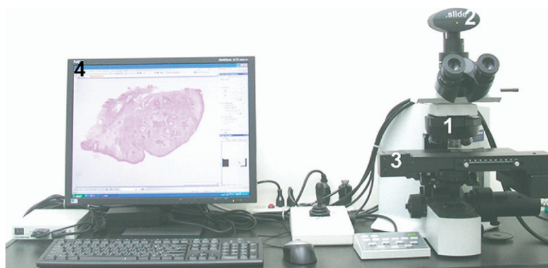
Fig. 1. The hardware used in the dot-slide system is chiefly composed of 1, a light microscope equipped with a motorized nosepiece; 2, a high-resolution digital color camera ( 1376 \times 1032 pixels); 3, a stage that is motorized in all 3 directions and can be moved with both the joystick and the software; and 4, a PC installed with the image acquisition software, with a monitor of standard resolution of 1600 \times 1200 dpi. The server computer is not shown.
