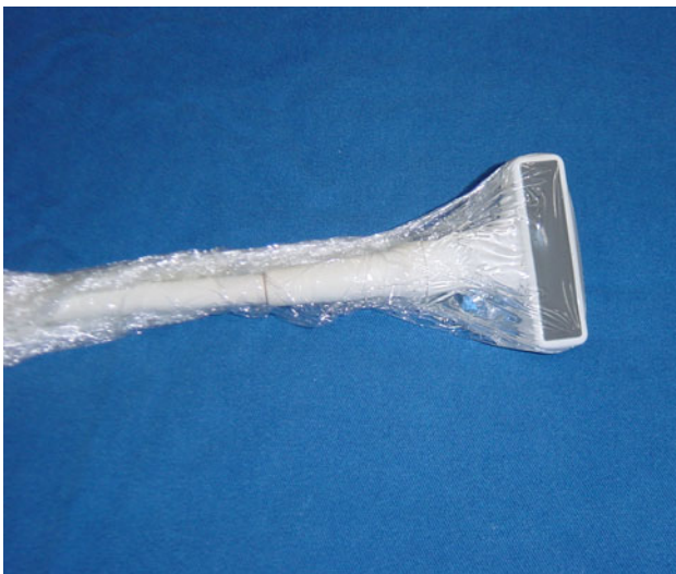
Fig. 1 High-frequency T-type linear array probe with lateral field-of-view, coated with sterile gel and covered with a rubber sheath
