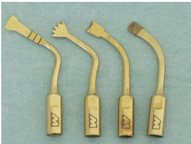
FIGURE 5. Bone saws are titanium nitride-coated inserts: it makes them hard enough to cut bone with the maximal power of the generator. These are 5-tipped saws and large-edged scalpels that can become real micrometric oscillating saws under the impulsion of intermediate frequency vibrations.
